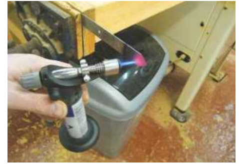
▲ Pic 7 He used a blow torch to heat and harden the steel of the blade, which was clamped in a vice
